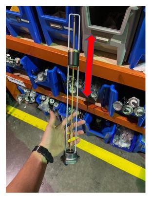
Reconnect the fuel sensor and manually add fuel. Check if your control panel indicates that fuel level is rising. If it is, then keep manually adding fuel until you reach 98% capacity.
