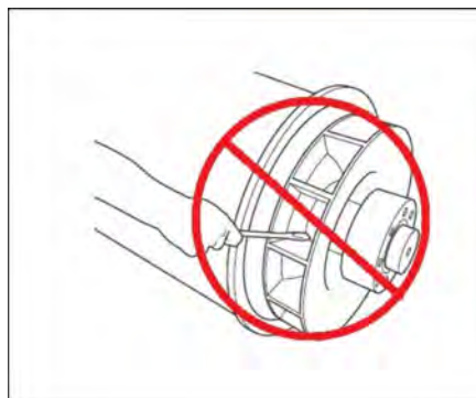
FIGURE 4. DO NOT ROTATE GENERATOR ROTOR WITH SCREWDRIVER
