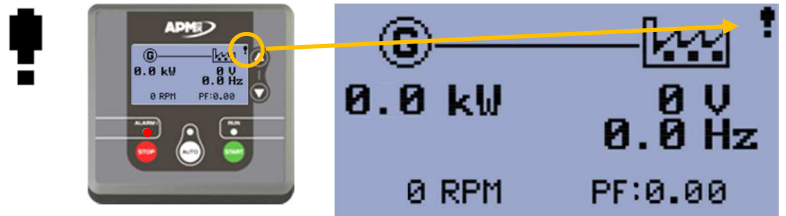
Figure 14 - appearance of a fault
