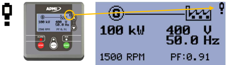
Figure 13 - appearance of an alarm
