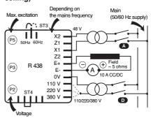
Static adjustment of the current limit, potentiometer P5 (factory setting: 7.5 A, fuse rating: 8 A - 10 seconds).
