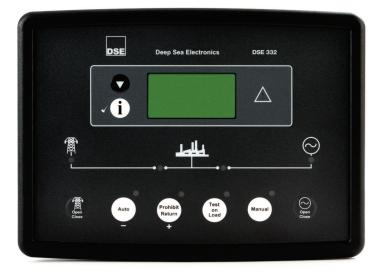
The DSE332 is an Automatic Transfer Switch Controller for single set genset applications. The module will monitor the voltage and frequency of the incoming AC mains (utility) supply (supports many topologies) and in the event of a failure will issue a start command to the generator control system.
