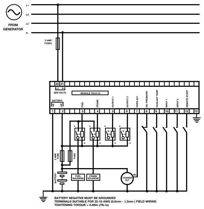
\* NOTE. ALL THE OUTPUTS ARE SOLID STATE AND ARE NEGATIVE SWITCHING
