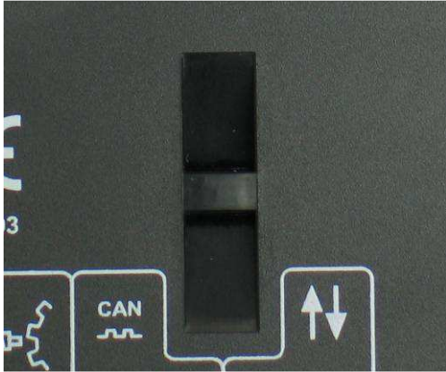
Cable tie fixing point
