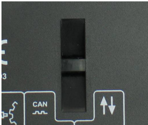
Cable tie fixing point
