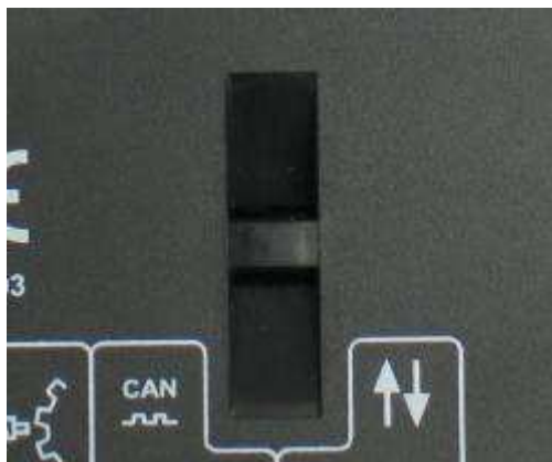
Cable tie fixing point
