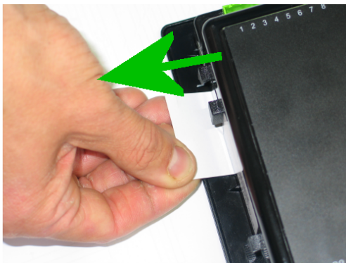
Removal and insertion of the LED text insert card
