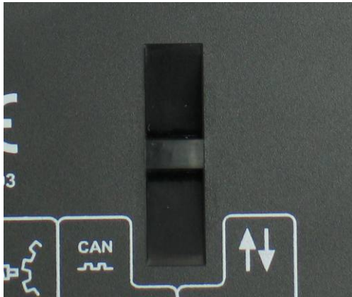
Cable tie fixing point
