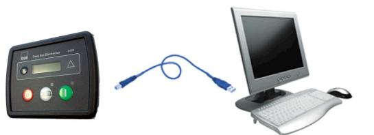
**ONOTE:-** The DC supply must be connected to the module for configuration by PC.
