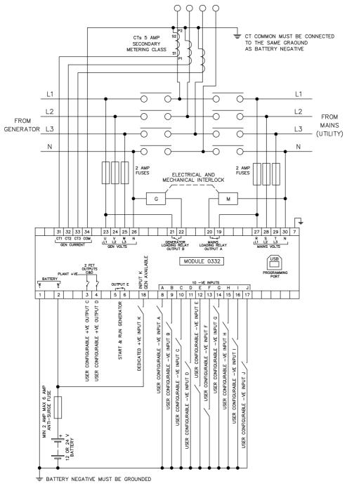
TERMINALS SUITABLE FOR 22-16 AWG (0.6mm - 1.3mm ) FIELD WIRING
