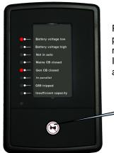
Pressing the button will signal to the host controller that the button is pressed. The controller will respond by lighting all LEDs on the 2548 module (lamp test) and silencing the sounder (alarm mute). If configured to do so, the host controller will also perform a lamp test and alarm mute function.
