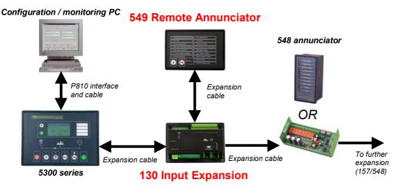
**NOTE:-** Previously, the 53xx expansion port was used solely for output expansion. For this reason, modules manufactured prior to the release of the P130 input expansion module may be marked as : 157/548 These 'early' modules are not compatible with the P130 input expansion module.
