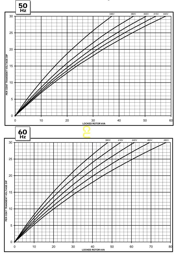
**PI144G** Winding 311 AS480 AVR With EBS fitted Locked Rotor Motor Starting Curves
