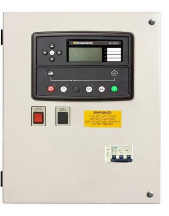
The panel is constructed in 1.5mm steel, powder coated to RAL9001 for a high quality, durable finish and mounted on a rigid stand. The generator circuit breaker is included within the box, together with all terminals for site interconnections.
