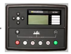
The BC 7320 control system (just the DSE7320 module is shown here) has an identical feature set to the BC 7310 but with the addition of full AMF functionality with integrated mains monitoring.
